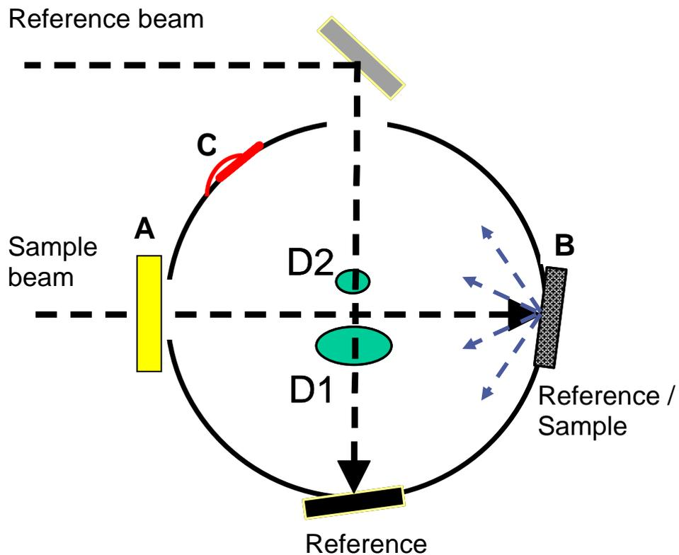
Figure 1. Experimental configuration for the measurement of spectral transmittance and reflectance (UV/Vis/NIR) using the PELA 150 integrating sphere reflectance accessory.
