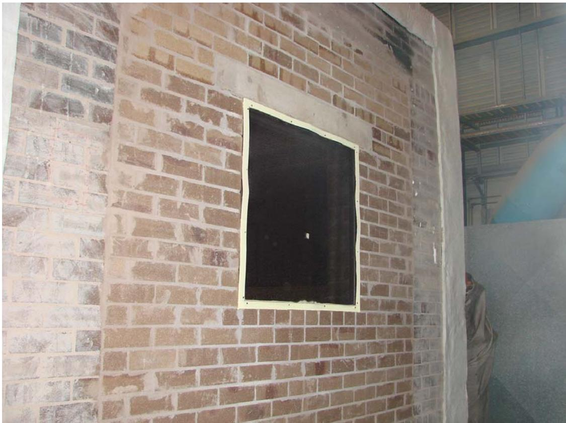
Photograph 8 - Exposed face of the specimen at the completion of testing
