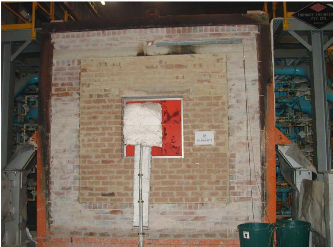
Photograph 4 - Specimen at 30 minutes into the test
