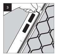
Cut spline and remove unwanted section.
