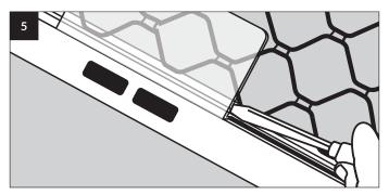
Place flat screwdriver under edge as shown and lever upwards.
