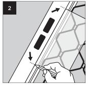
Place "ProwlerGuard" in required position and mark where to cut the spline
